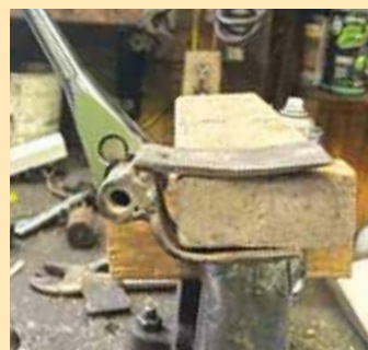
Shortridge used the two ends of a bar to make the jaws, one with a 90-degree curve and the other with a slight curve. He welded them together with both curves in parallel, placing a socket on the back side of the clevis.
