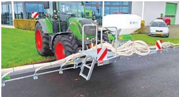
Booms are available in three widths, and units can be folded either mechanically or hydraulically.
