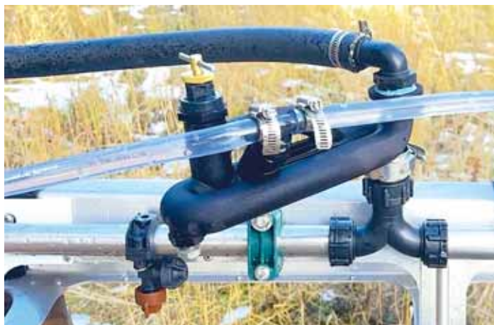
The core of the system is the Sectional Recirculation Valve, which directs product through each boom and returns it through a polyethylene-lined return line.
