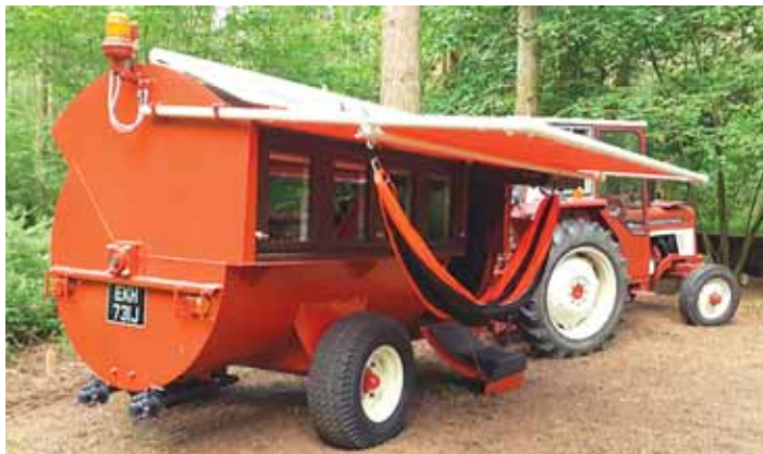
Camper has hot and cold running water, a luxurious wooden interior, numerous electronically actuated devices, and an exterior safety beacon that folds down to reveal a showerhead.
