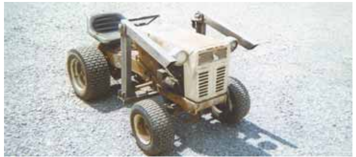
After removing the mower deck, Hileman used its drive belt to operate a new hydraulic pump that powers the loader.
