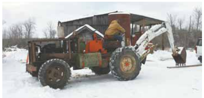
An old backhoe mounted on back of a stripped-down Case combine does heavy duty work for Roger Lindbeck. It also uses the engine and steering wheels from a 1 1/2-ton Ford truck.
