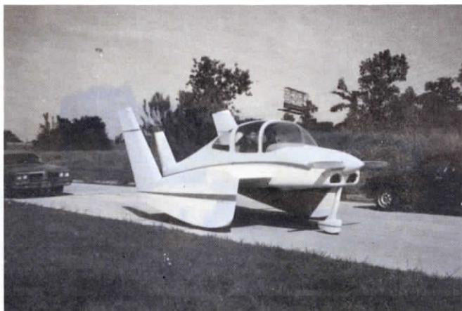
Wernicke's Aircar has a short 10-ft. wingspan. Top air speed will be 266 mph.
